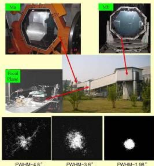
From 2001 to 2004, an experiment equipment built in Nanjing was been using for testing of thin mirror active optics.
