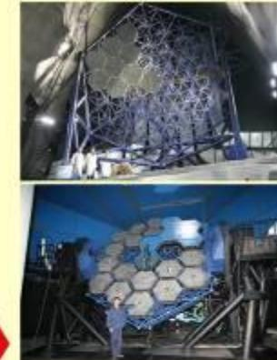
In May of 2007, a small system of LAMOST was finished. It has 6 Ma and 9 Mb sub-mirrors with aperture of 2 meters, a small focal plane with field of view of 1.2 degrees, a small fiber positioning system with 250 fibers, and the first spectrograph with two  $4 \times 4$  k CCD cameras.
